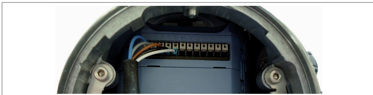
Fig. 24: Wiring of the 12 push-in terminal strip
